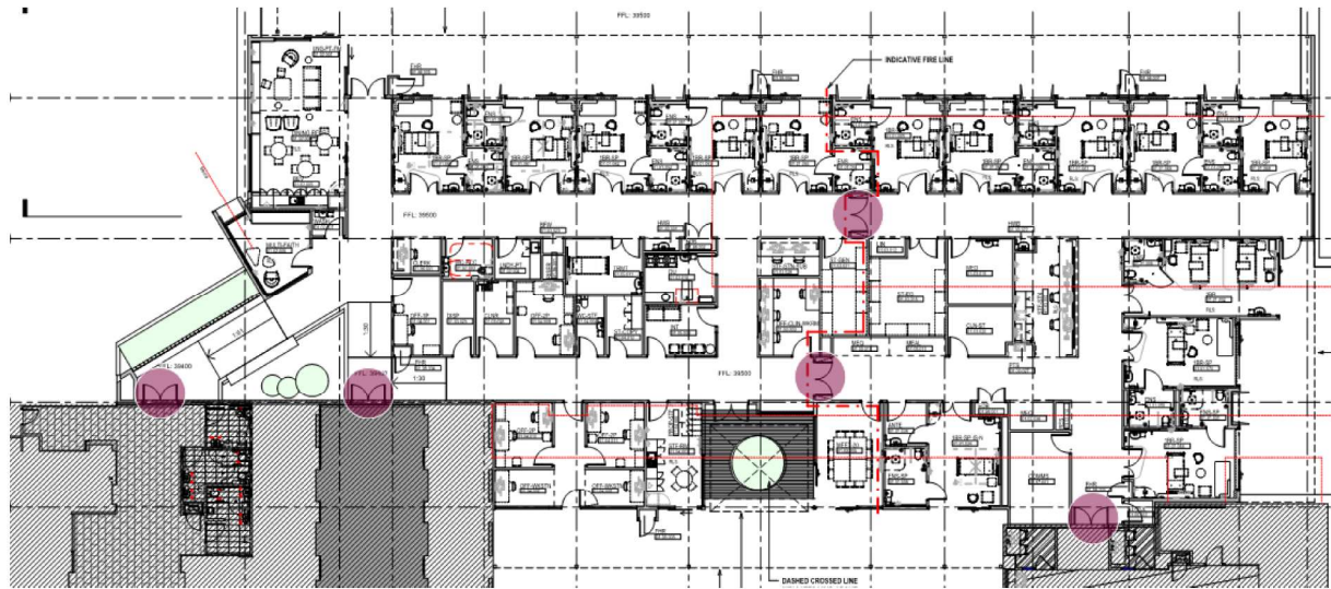
Figure No. 17: Horizontal exit doors that do not swing in the direction of egress
